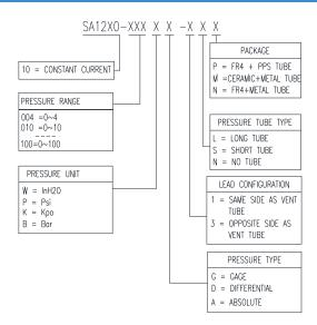
Part Number Example: SA1210-005WD-3SM 0~5 InH2O Differential, Short Metal Tube, Pins Down, SA12 Product
